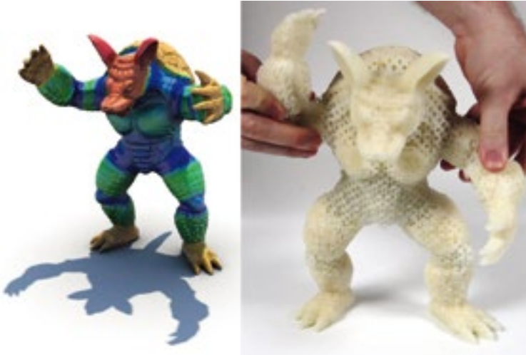
Assemblage of microstructures that approximates the desired elastic behavior and requires only a single material for fabrication.
