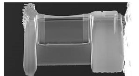
SEM of a TEM lamella after the thinning procedure. The cross section will be analyzed in the TEM at the EM Facility
