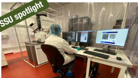
Helios G4 dual beam Xe FIB – UHR SEM installed in the I21 LBW
